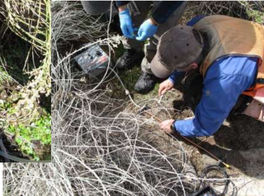
Collection of He sample in copper tubing
